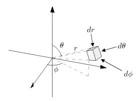
The cell includes the volume lying between r and r+dr, between  $\theta$  and  $\theta+d\theta$ , and between  $\phi$  and  $\phi+d\phi$ . In the limit as dr,  $d\theta$ , and  $d\phi$  all approach zero, the cell approaches a rectangular solid with sides of length:
