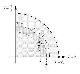
Note that the strip has a coordinate width of dr, but the distance across the width of the strip is determined by the metric to be
