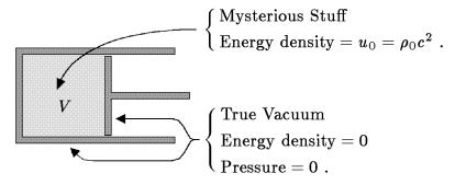
The piston is then pulled outward, so that its initial volume V is increased to  $V + \Delta V$ . You may consider  $\Delta V$  to be infinitesimal, so  $\Delta V^2$  can be neglected.
