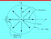
The fraction of the photons hitting the sphere that hit the detector is just the ratio of the areas:
