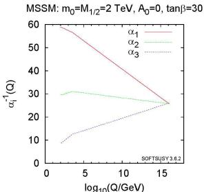
The top graph shows the running of coupling constants in the standard model, showing that the three coupling constants do not quite meet. The bottom graph shows the running of coupling constants in the MSSM — the Minimal Supersymmetric Standard Model, in which the meeting of the couplings is almost perfect.  $\alpha_i = g_i^2/4\pi$ .
