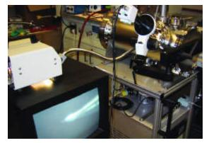
**Figure 6:** The SPL small vacuum facility for colloid research. The microscope display is showing the tip of a cone-jet emitter in operation.
