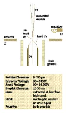
Figure 4: Basic principle of operation of a colloid emitter
