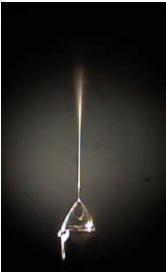
**Figure 5:** Cone-jet structure in the laboratory. The liquid used had low conductivity, which allowed the jet to be large enough to be visible. With more concentrated solutions, the jet diameter is smaller than the wavelength of light and becomes invisible.
