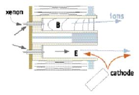
**Figure 1:** Schematic of a Hall thruster. The annular channel is ceramic lined. A plasma forms near the exit plane, where the magnetic field, B, is maximum. Ions accelerate electrostatically in an electron-neutralized background, and no grids are necessary.
