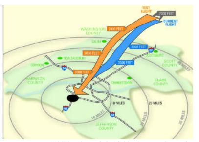
Standard flight paths at Louisville (blue) involve a series of staggered descents producing significant noise from multiple thrust increases and landing-configured aircraft systems. The test past (orange) keeps aircraft higher, longer. (Drawing adapted from a Convington Journal Illustration by Mike Covington)
