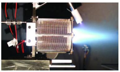
**Figure 2:** A 200W Hall thruster (courtesy Busek Co. Inc.) in the 1.5X1.5 m vacuum chamber at the SPL. The blue light is mainly from excited Xe ions in the plume. The device at the top is the neutralizing hollow cathode.
