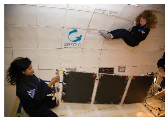
Aboard the Zero G flight, Tina Srivastava (left) and Jillian James test microgravity deployment of a solar panel for an undergrad satellite project. (Steve Boxal/Zero Gravity Corp. photo)
