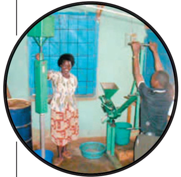
The Approtec Oilseed Press in Use in Kenya
