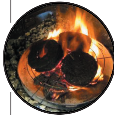
Hand formed briquettes crumble upon burning and are unable to boil water for as long as wood charcoal.
