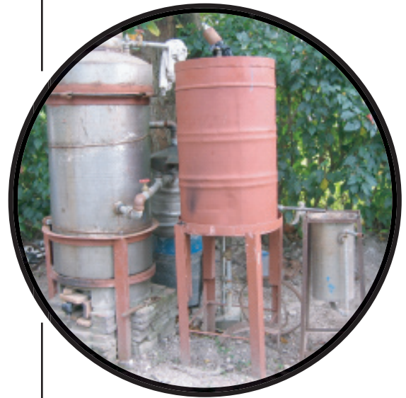
A distillation system used in Haiti currently. From left to right are shown the steam generator, condenser, and separator.
