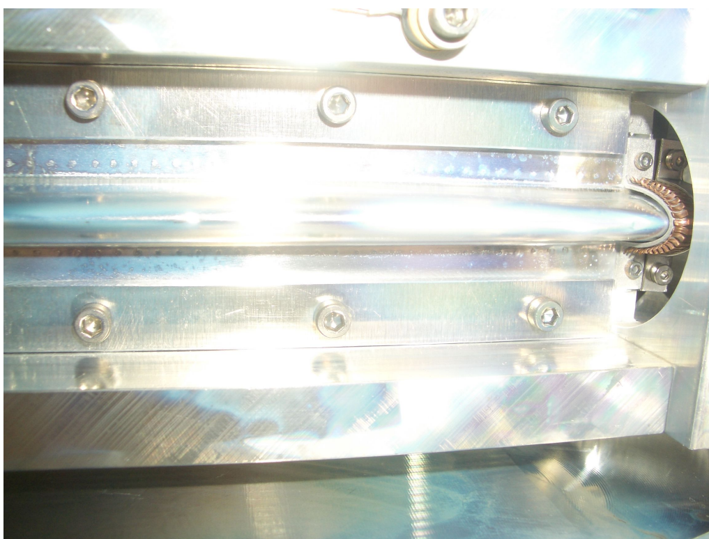
Cell wall not attached to the aluminium ring anymore.
