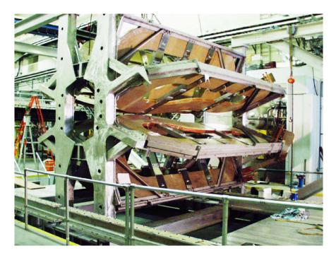
Figure 2.4: The eight coil BLAST toroid without its detectors.
