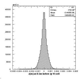
Origin of electrons hitting fixed collimator
