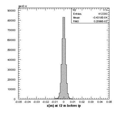
Horizontal and vertical distribution of electrons after fixed collimator 0.5m in front of IP
