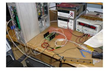
3 stage readout electronics (ADC, supply board, APV board)
