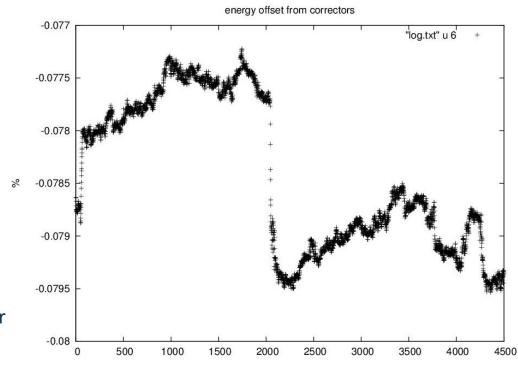
Effect of correctors calculated over 12 hours during a 4.5 GeV run: 2 x E-5
