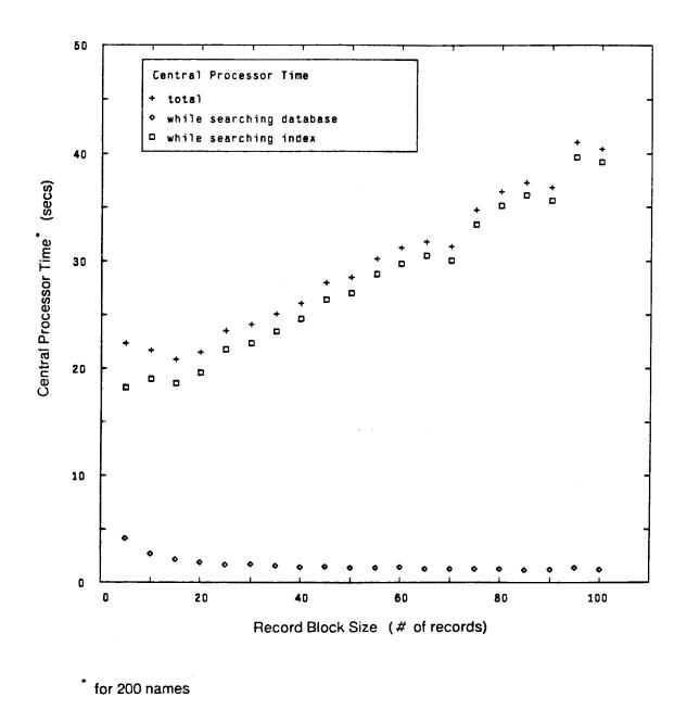
Figure B-10: Central Processor Time vs. Record Block Size, Buffer Size 2048
