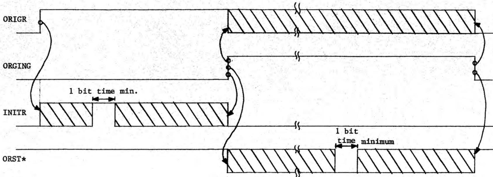
Figure 3 -- Initialize and Reset Mode Timing
