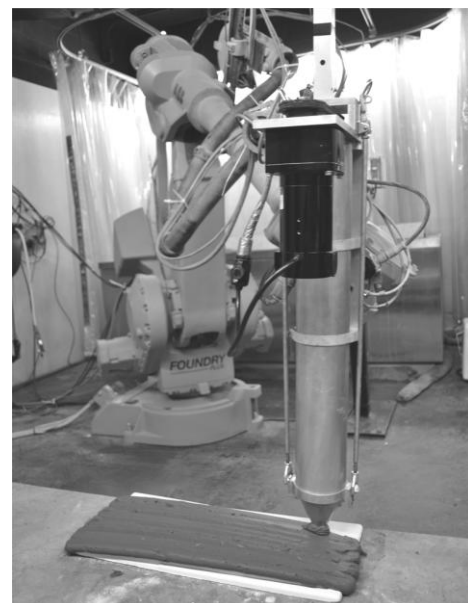
Fig. 7 Ceramic deposition in progress
