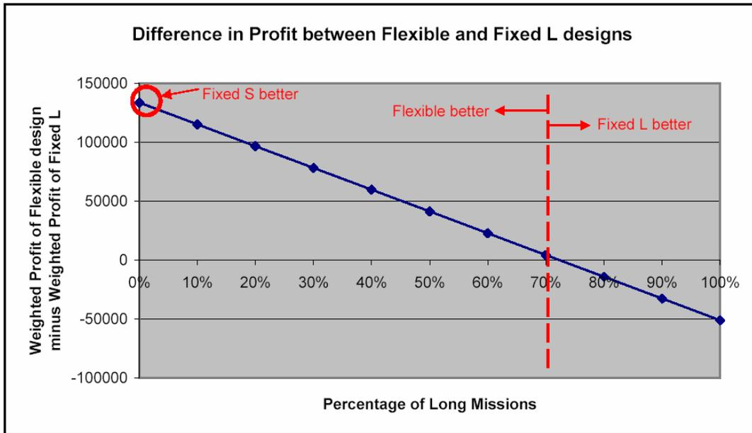
**Figure 4 Difference in weighted average profit between flexible and Fixed L designs. Break-even point occurs at 70% long duration missions.**
