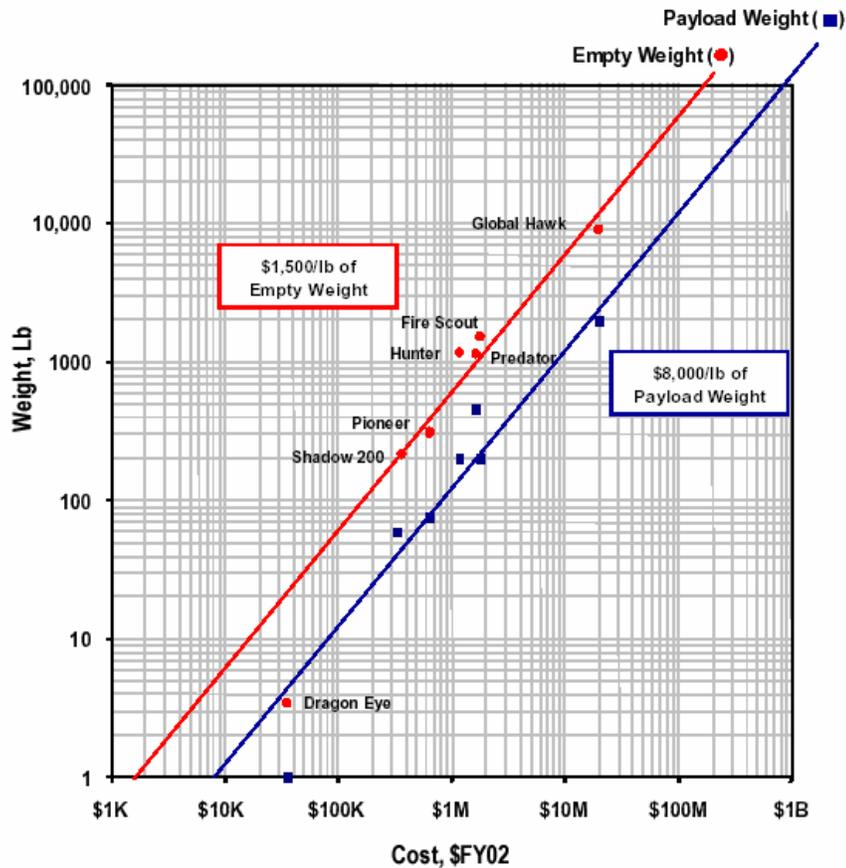
Figure 3 Cost versus weight of uninhabited air vehicles. (Source: [http://www.uavforum.com/library/uav\\_roadmap\\_2005.pdf](http://www.uavforum.com/library/uav_roadmap_2005.pdf))
