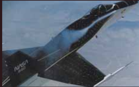
A flight test of the F/A-18 shows the dispersion of smoke particles that results from a vortex burst (left). Automatic identification and visualization of vortex cores, developed by Aero-Astro's Robert Haines and Dr. David Kenwright of NASA Ames, reveal the same behavior in a CFD simulation (right). Visualization software developed by Haines is used throughout the world.
