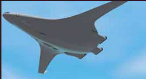
The Aero-Astro/Cambridge University Silent Aircraft Initiative was conceived to make a substantial reduction in aircraft noise. The plane could also reduce fuel consumption by 25 percent compared to current aircraft.
