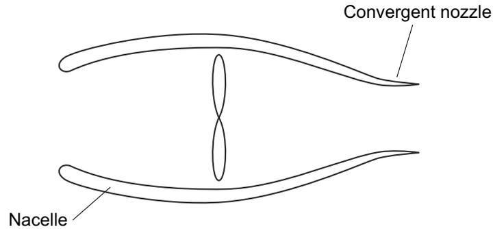
Figure 4: Propulsor-nozzle configuration: convergent nozzle.
