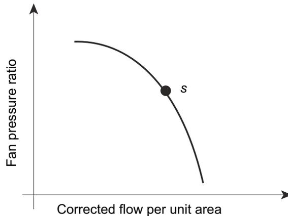
Figure 5: Fan pressure ratio versus corrected flow per unit area.
