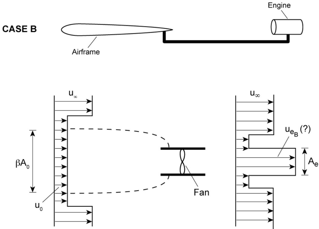
**Expanded view of ingested wake and fan inside the engine for Case B**
