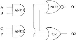
The inputs to the flux capacitor, A, B, C, D are all true, and the outputs O1 and O2 are also both high. Let us determine if this is a fault condition, and which components may have failed.
