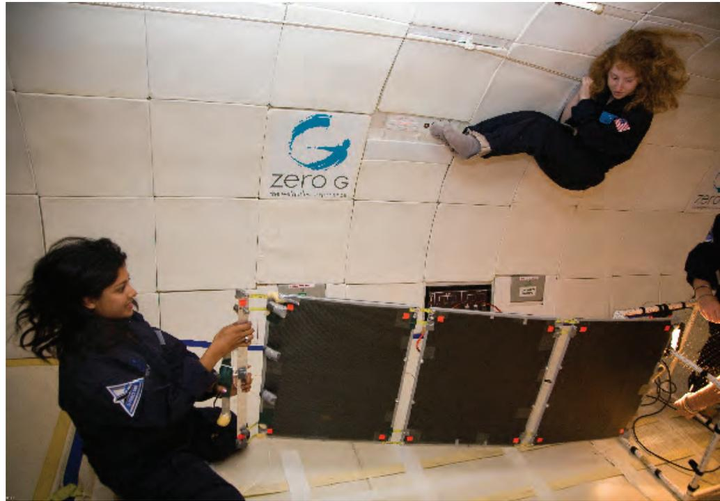
Aboard the Zero G flight, Tina Srivastava (left) and Jillian James test microgravity deployment of a solar panel for an undergrad satellite project. (Steve Boxal/Zero Gravity Corp. photo)
