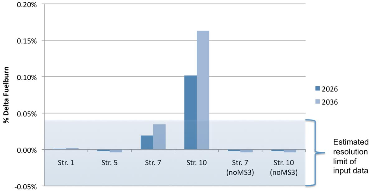
Figure 21: Climate Inputs; % Change in Full Flight Fuel Burn (large engines only)
