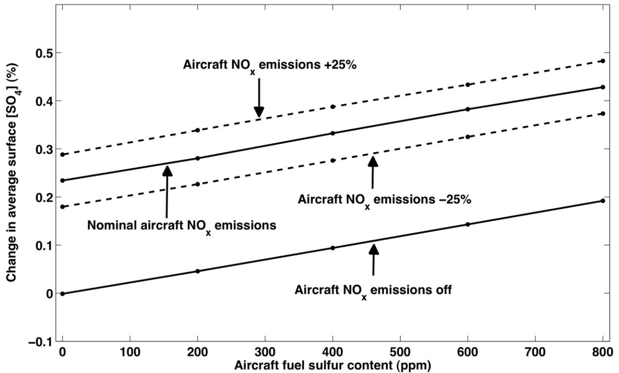
**Figure 12: Relative change in average surface sulfate concentration attributable to aircraft emissions as a function of assumed fuel sulfur content for aircraft NO<sub>x</sub> emissions at their nominal value, perturbed by ±25%, and switched off. Results from 20 GEOS-Chem full year calculations are shown.**
