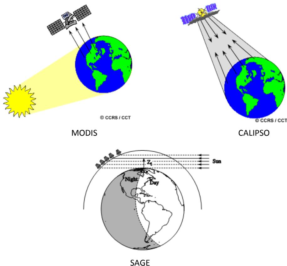
**Figure 1. Schematics of MODIS (passive, total column) (Natural Resources Canada, 2012), CALIPSO (active, vertically resolved) (Natural Resources Canada, 2012), and SAGE (passive, vertically resolved) (NASA, 2004) retrievals.**
