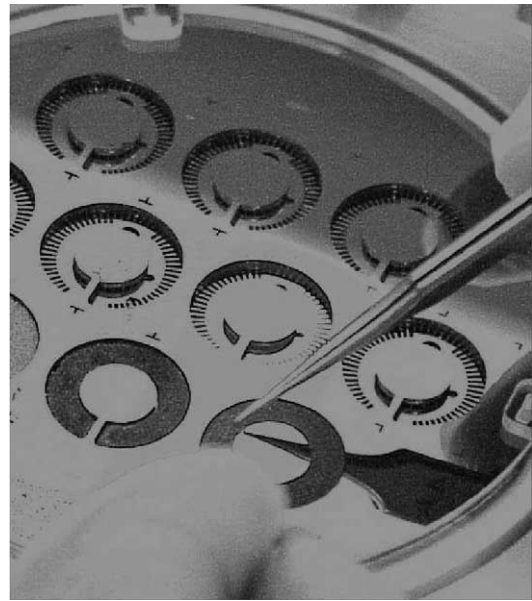
Fig. 5. Catalytic pieces being inserted into six-wafer combustor during fabrication.
