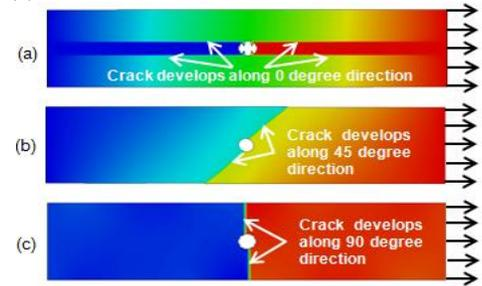
**Figure 2:** Sharp (strong-discontinuity) crack obtained with the novel method for open hole tensile loading of lamina for three cases of fiber orientation (a) 0 degree, (b) 45 degree, (c) 90 degree
