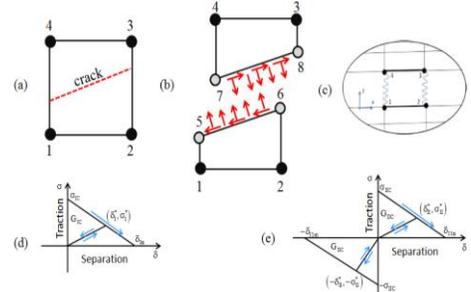
**Figure 1:** (a) Continuum element, (b) Element splitting due to crack, (c) Cohesive zone modeling, (d) Mode-I cohesive law, (e) Mode-II cohesive law
