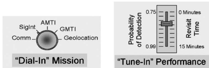
Fig. 11. Two generic types of flexibility: The ability to modify the mode of operation of a system (dial-in mission), and the ability to modify the attribute of a requirement (tune-in performance).
