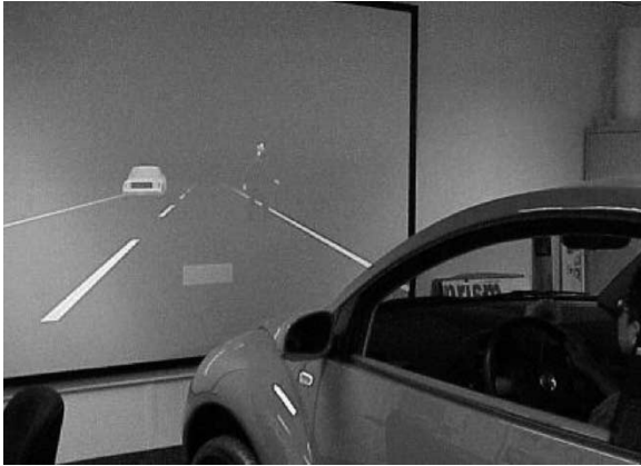
Fig. 1. Experimental setup. A warning to indicate the existence of a pedestrian was provided visually to the driver using a simulated head-up display.
