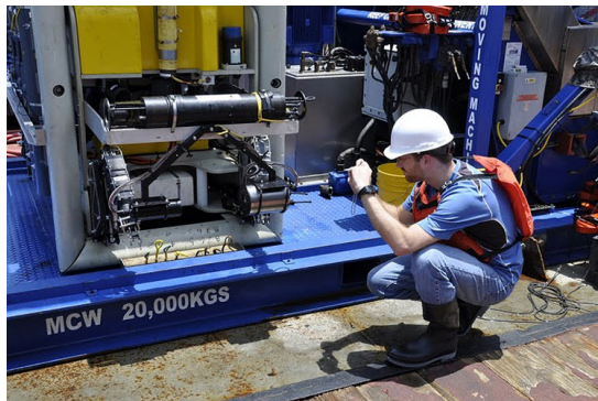
MIT/WHOI Joint Program graduate student Nick Loomis viewing a digital holographic instrument mounted on a remotely operated underwater vehicle to study the oil spill in the Gulf of Mexico in June 2010.
