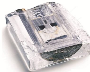
Figure 1. A prototype of the liquid metal battery. The cutaway shows the three layers. Courtesy Sadoway lab.
