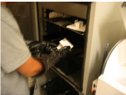
Step 11 – Dip model in wax after de-powder let dry on shelf for 1 hour
