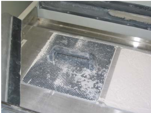
Step 17 – Set surfaces for feed and build. * The build must be at the top (Empty)
