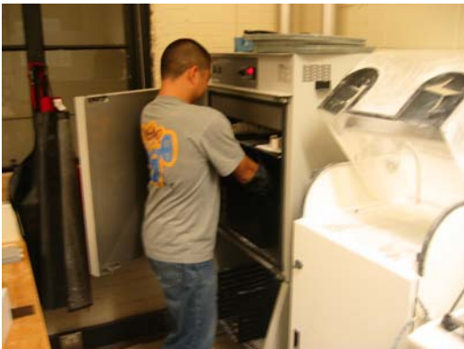
Step 11 – Dip model in wax after de-powder let dry on shelf for 1 hour
