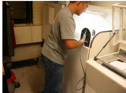
Step 12 – Reset machine, place powder from over flow into the feed
