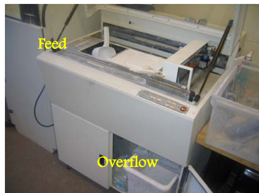
Step 12 – Reset machine, place powder from over flow into the feed
