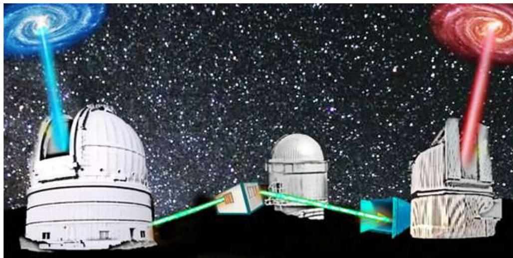
Schematic of the 2018 "Cosmic Bell" experiment at the Roque de Los Muchachos Observatory in the Canary Islands, where two large telescopes observed the fluctuating color of light from distant quasars (red and blue galaxies). The green beams indicate polarization-entangled photons sent through the open air between stations separated by about one kilometer. Credit: Andrew S. Friedman and Dominik Rauch
