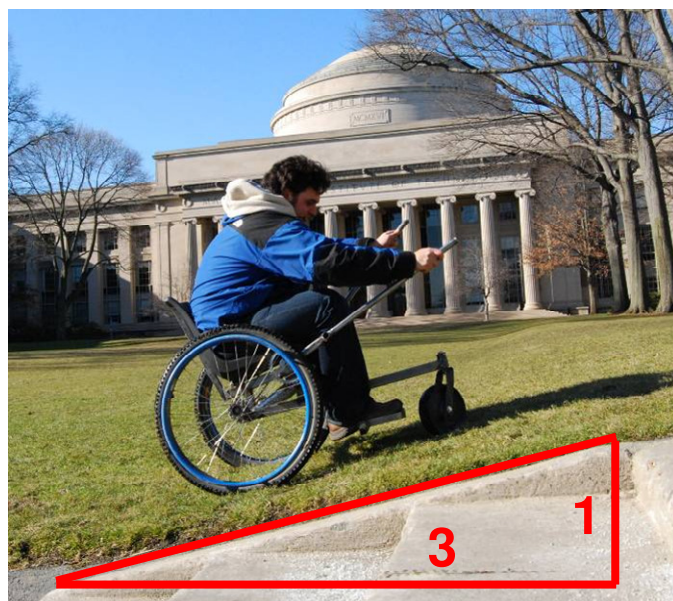
Figure 11. LFC going up 1:3 rise during hill climb trials
