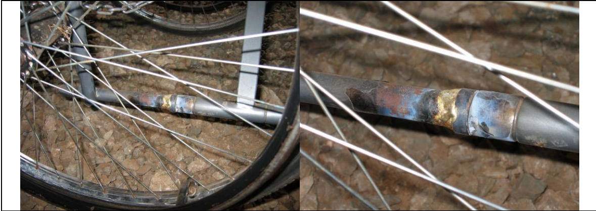
Figure 2.17 Cracked weldment on bottom tube of WTTC 4-wheeler
