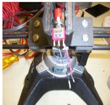
A: Vertical thruster interconnecting wires
