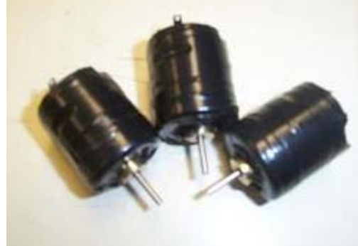
Figure 8: 12VDC Motors sealed with electrical tape
