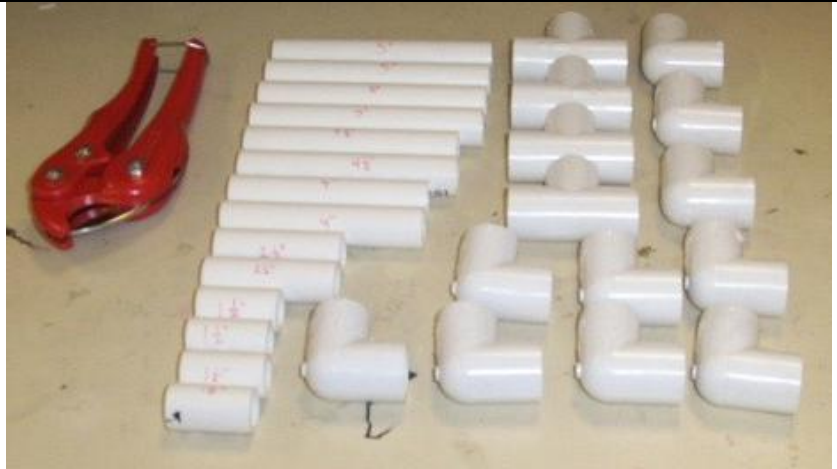
Figure 1: PVC pipe cutter, Cut sections of PVC pipe, Elbows and T's
