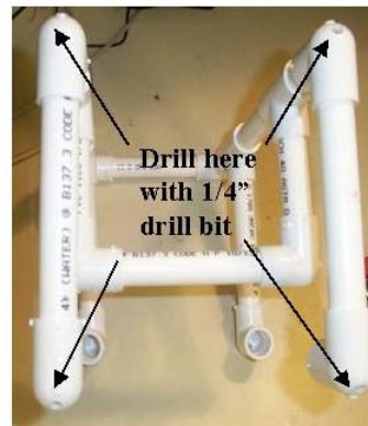
Figure 3: Drain holes in elbows drilled with 1 / 4" drill bit
