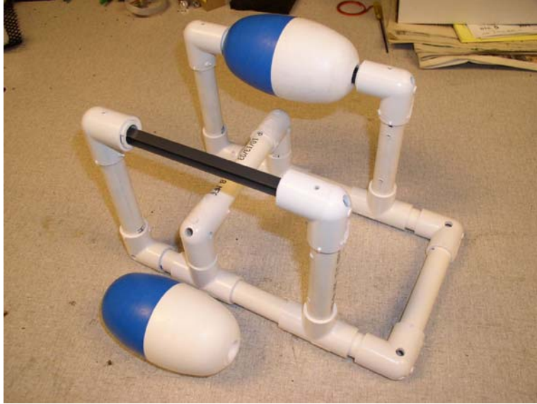
Figure 4: H-beam Assembly for floats
