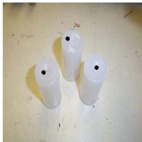
A: Film cans drilled with 3/32" drill bit
