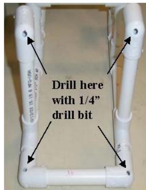
Figure 3: Drain holes in elbows drilled with 1 / 4" drill bit
