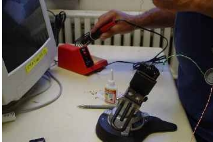
Figure 10C: Tether wire soldered to motor
