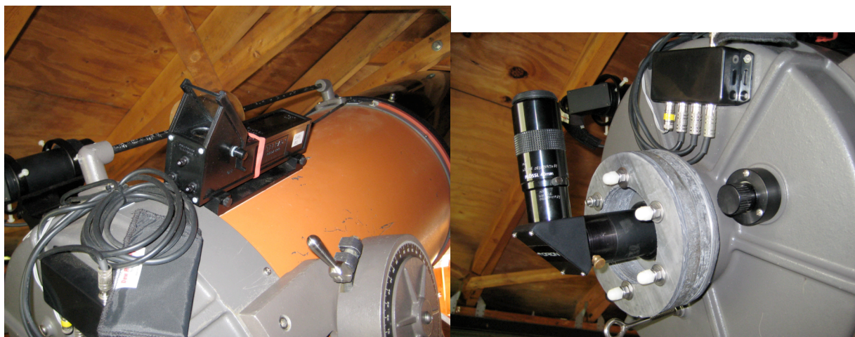
Figure 19. 14-inch Celestron telescope with Telrad (right), and with 40mm Plossl eyepiece (left)
