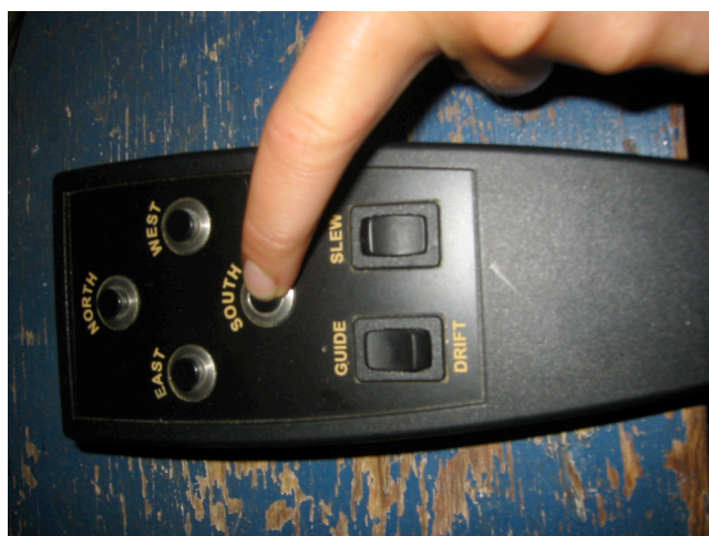
Figure 28. TCS handpaddle. Use the directional buttons to move the telescope, and the Guide/Drift/Slew buttons to adjust the rate.
