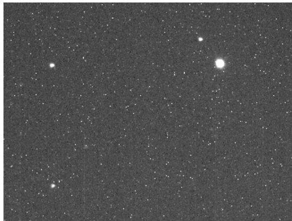
Figure 39. Focused image before calibration. This image was taken after focusing the CCD. You can tell that the image is well-focused because the target and three comparison stars now all appear as sharp images rather than doughnuts. The fainter blemishes are more distant stars, while the white speckles are again, hot pixels, and will be removed upon calibration. If you look closely enough, you will be able to see the same hot pixel patterns in this image with the uncalibrated image on the previous page.
