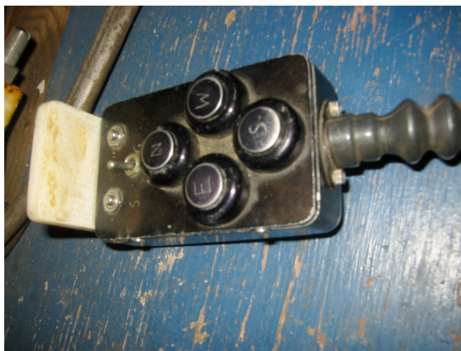
Figure 27. Focus controller. The two buttons to the left in this picture will move the focuser.
