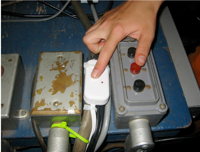
Figure 25. Dome rotation controls. The white slider will turn on a light that illuminates the dome numbers. The black buttons on the grey controller move the dome, and the red button stops the rotation.
