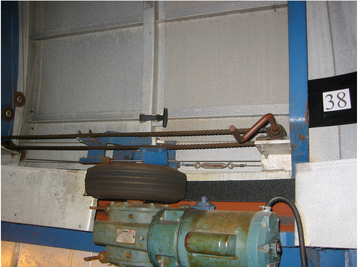
Figure 23. Dome shutter. Open by releasing the rubber latch in the center, and cranking the handle on the right.
