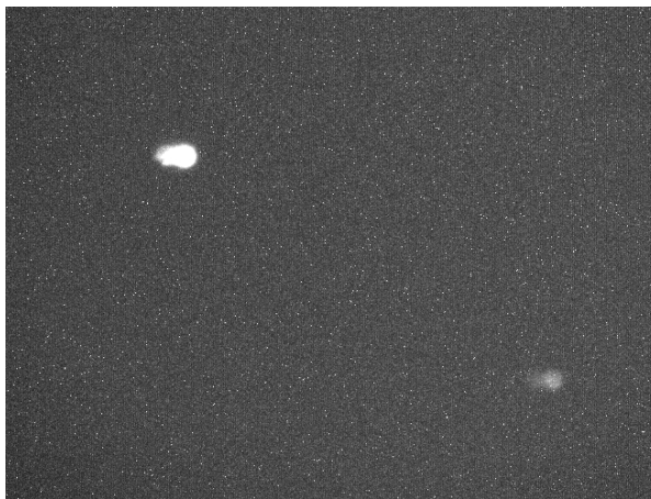
Figure 43. Data taken on Sep. 28, 2006 at 02:25 UT. Asteroid Iris and a comparison star. Trailing due to bumping of the telescope while it was taking an exposure, on Telescope 2 (an automated GO-TO telescope), producing double images.
