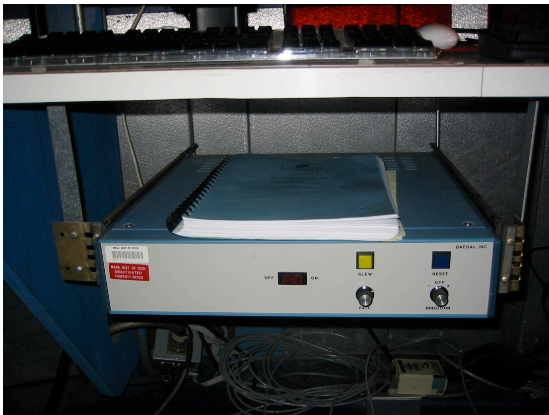
Figure 26. DAEDAL controller. This only needs to be turned on during focusing.
