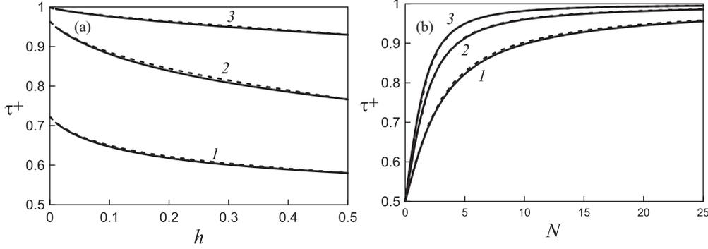
FIG. 5. (a)  $\tau^+$  versus channel width  $h$  for  $N = 1$  (1),  $N = 5$  (2), and  $N = 25$  (3); and (b)  $\tau^+$  versus  $N$  for  $h = 0.25$  (1),  $h = 0.05$  (2), and  $h = 0.01$  (3).  $\tau^+$  determined from the model (27)–(60) (continuous line) and  $\tau^+$  computed numerically in the full 2D model near equilibrium (dashed line).
