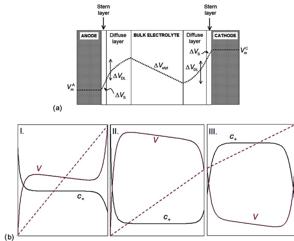
**Figure 1.** (Color online) (a) Schematic representation of the electrostatic potential profile in the fuel cell membrane. In this representation, there is an excess of protons in the anodic polarization layer and a deficit on the cathodic side. (b) As in (a), but for three cases: I, as in (a); II, with an excess of protons on both sides; and III, with a deficit of protons on both sides. The dashed lines show the electrical voltage increase through the external circuit.
