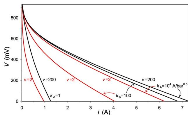
**Figure 6.** (Color online) Influence of proton volume constraints on the generated cell voltage  $V$  as function of current  $i$  ( $\delta = 1$ ,  $k_C = 10^4 \text{ A/bar}^{1/2}$ ,  $R_{\text{elyt}} = 68.9 \text{ m}\Omega$ ).
