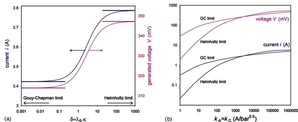
**Figure 4.** (Color online) Influence of  $\delta$ , the ratio of Stern layer thickness  $\lambda_S$  to the diffuse-layer thickness,  $\kappa^{-1}$ , on concentration-cell current  $i$  and voltage  $V$ . (a) Continuous curves are based on full calculations; the Helmholtz limit is based on Eq. 25, and the GC limit on Eq. 27.  $k_A = k_C = 10^4$  A/bar<sup>1/2</sup>. (b) Results for  $i$  and  $V$  in the GC and Helmholtz limit as a function of  $k_A = k_C$ .
