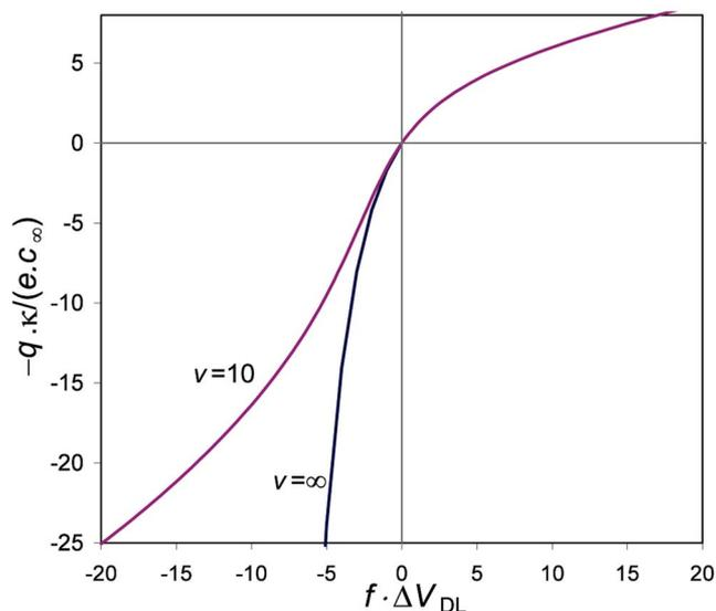
**Figure 2.** (Color online) Surface charge density  $q$  of the polarization layer as a function of diffuse-layer potential difference  $\Delta V_{DL}$  according to the modified one-dimensional planar PB model with fixed anions and mobile cations, as function of volume parameter  $v$ , which is the inverse volume fraction of protons in the bulk phase.
