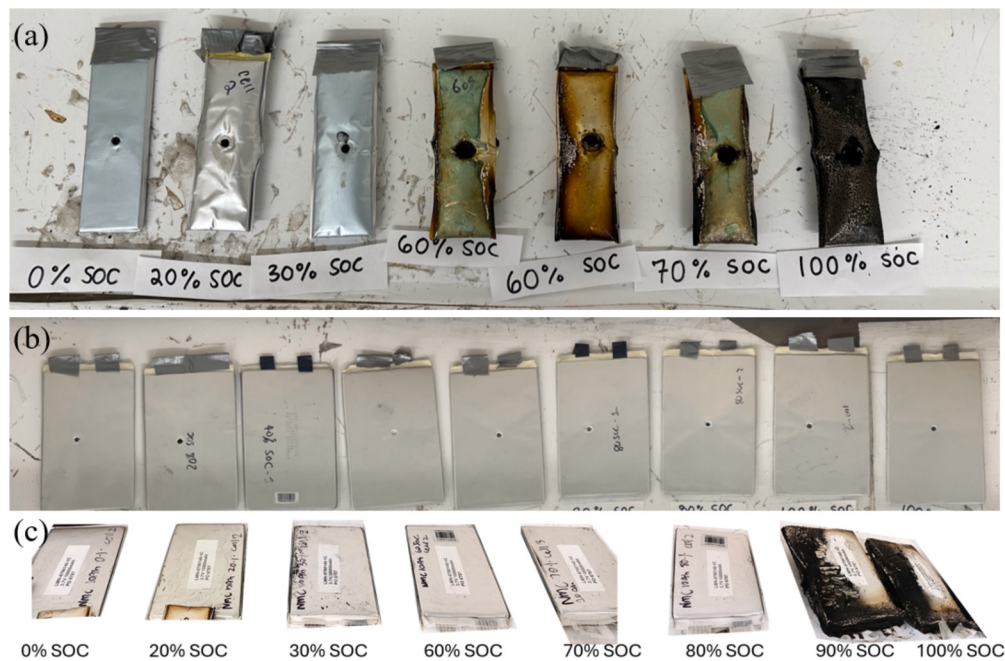
Fig. 9. Cells after indentation test, (a) LCO 4 Ah cells, (b) LFP 15 Ah cells, (c) NMC 10 Ah cells.
