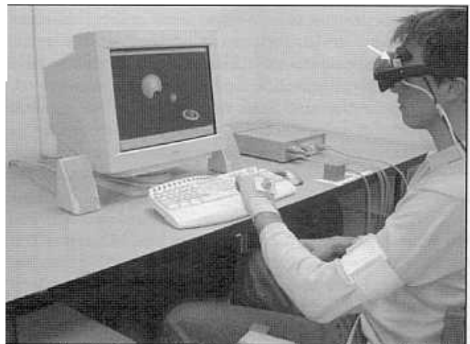
Figure 3. Head-mounted display consists of 2 mini displays mounted directly in front of the eyes, which provides a stronger sense of stereo separation. Head position and orientation collected by a magnetic sensor (arrow) change the viewpoint of the scene displayed by the VE software to compensate for head movement. Since the subject can only see what the HMD displays, the computer monitor can be used by the therapist to view what the patient is seeing without having to wear the equipment, if a dual monitor video card is used.
