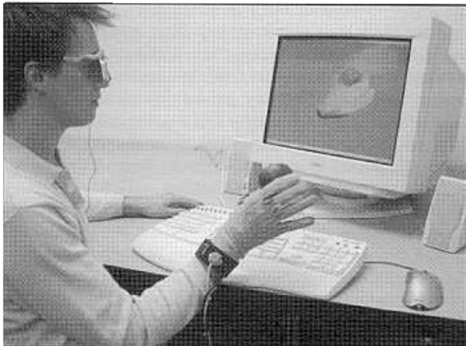
Figure 2. Subject is wearing 'flicker glasses' that induce a depth illusion in the viewed scene. The liquid crystal panels in front of each eye rapidly darken in synchronization with the display of left and right side images generated by the VE software, ensuring that each eye sees the appropriate images. Cyberglove on hand transmits hand and finger joint positions and orientations using fiber optic cables and a magnetic tracking sensor as described in Figure 1. Subject is also holding a 'real' object, which corresponds to a held object in the virtual environment to increase the sense of immersion and to elicit natural movements.
