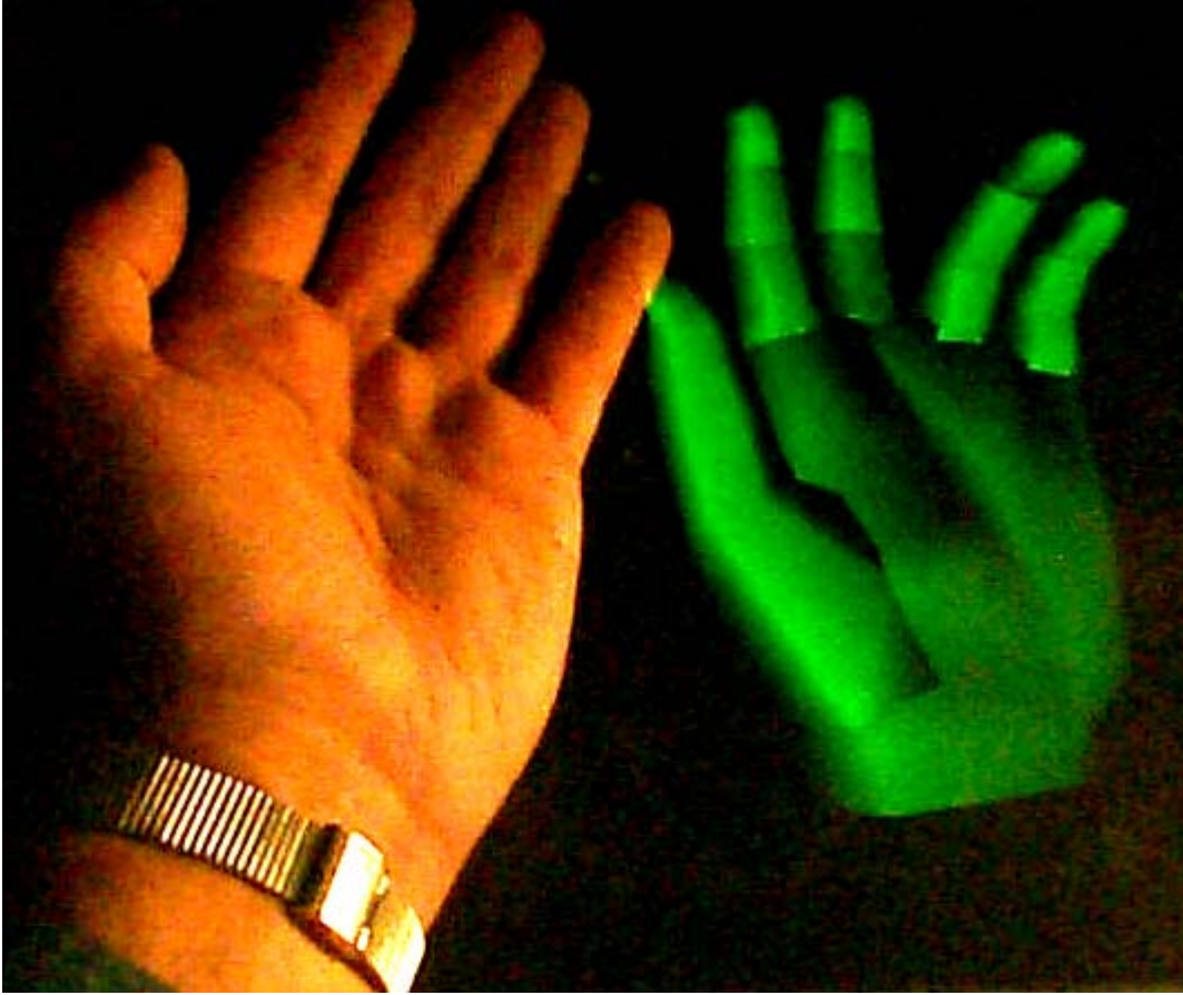
Figure 1. A photograph taken from the user's point of view, while the user is looking down through a semitransparent horizontal mirror. A monitor mounted above the mirror (facing down) projects virtual images, that appear aligned with the physical hand in the same workspace. Note that appropriate illumination has to be used in order to see both hands.
