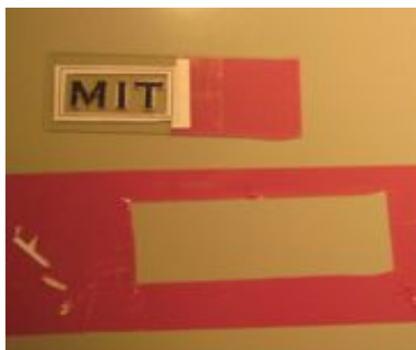
Students fabricated electrochromic devices out of M13 phage in the third module of 20.109, Fall 2007.
