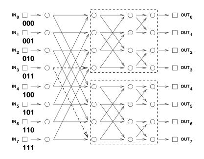
Despite the relatively complicated structure of the butterfly, there is a simple way to route packets. In particular, suppose that we want to send a packet from input  $x_1x_2...x_{\log N}$  to output  $y_1y_2...y_{\log N}$ . (Here we are specifying the input and output numbers in binary.) Roughly, the plan is to "correct" the first bit by level 1, correct the second bit by level 2,
