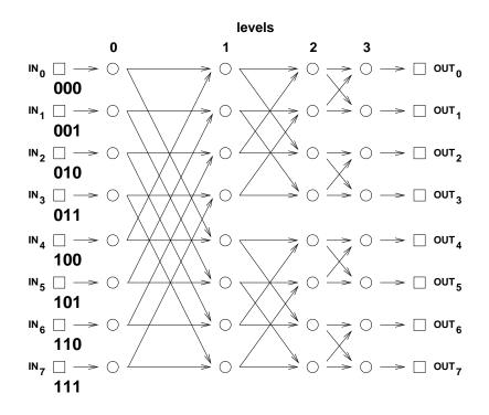
The structure of the butterfly is certainly more complicated than that of the complete binary tree or 2-D array! Let's work through the various parts of the butterfly.
