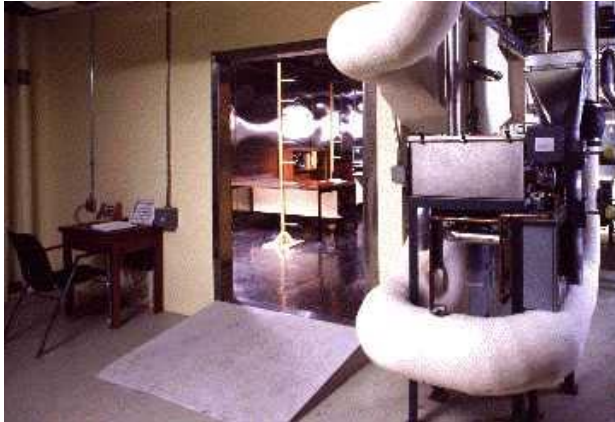
A large-scale stainless-steel chamber used to test material emissions.
