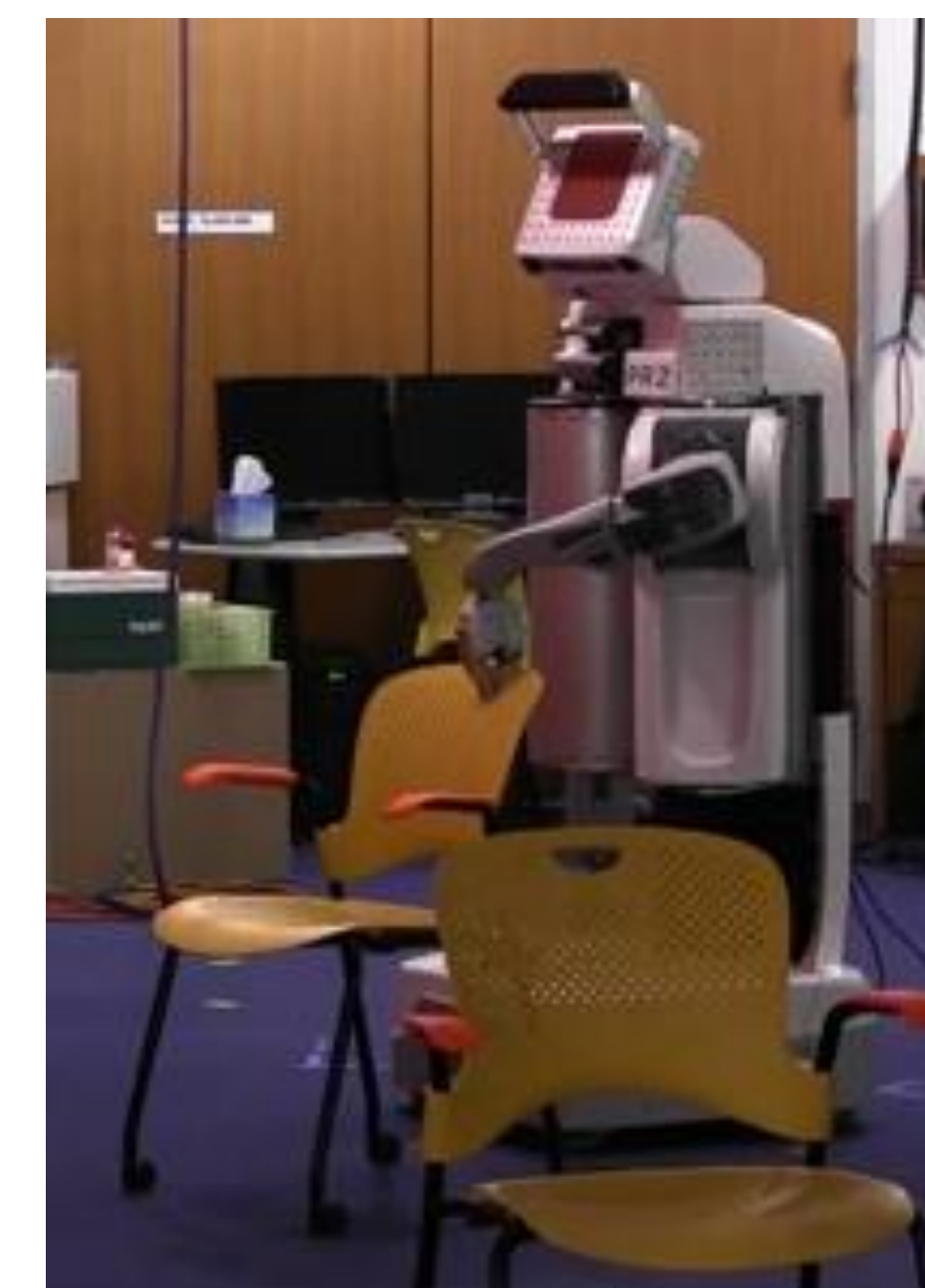
PR2 robot placing a chair Because chairs are comparable in size to the robot, bad placements can affect the robot's movement
