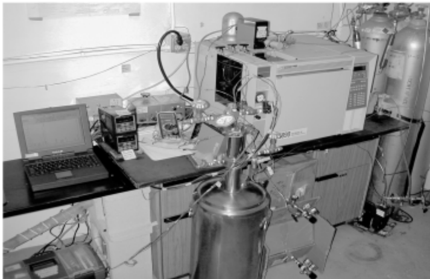
Figure A1. Halocarbon Detection System at Nahant, MA. Instrumentation includes automated cryogenic collection system (in the foreground) coupled with a Hewlett-Packard Series II Gas Chromatograph with Electron Capture Detector (on the bench).
