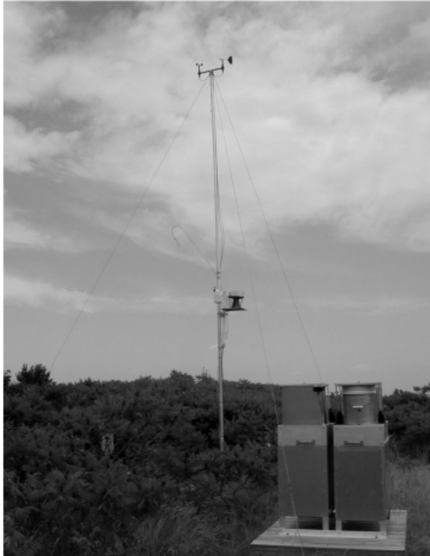
Figure A3. Air inlet on the roof of the bunker. \frac{1}{4} " stainless steel tubing extends from the laboratory up through a ventilation shaft to this meteorological instrument tower. Our air inlet can be seen extending out to the left just over halfway up the tower. A teflon funnel is inverted at the end of the stainless steel tube to prevent water from being sucked into the tube.
