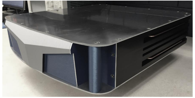
Fig. 2: A sample Power Electronics Building Block (PEBB) [3]. The top and/or bottom surfaces are available for transferring heat out of the unit.
