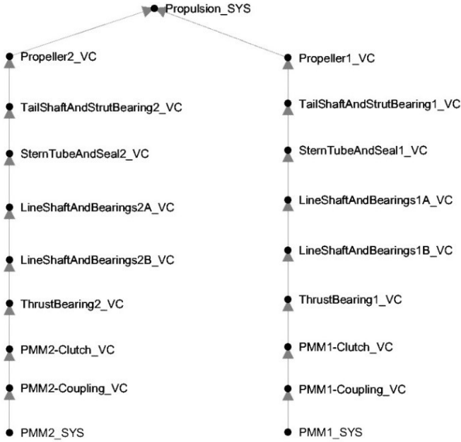
Fig. 3. Mechanical (Propulsion) Subsystem or Plex Logical Architecture (PMM in this figure stands for Propulsion Motor Module)
